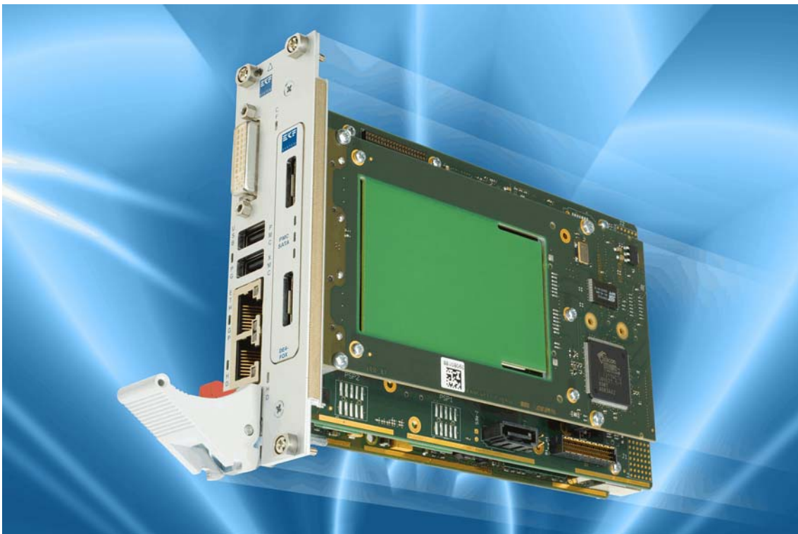
Assembly Stack: CCG-RUMBA (CPU) - CCK-MARIMBA (PMC Carrier) - DE4-FOX
